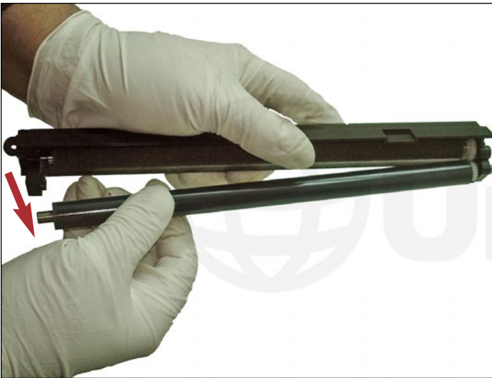
13. To remove the PCR, press it toward the gear to loosen the other end, and take it out from the assembly.
