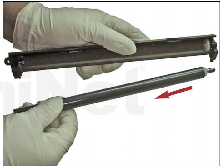
13. To remove the PCR, press it toward the gear to loosen the other end, and take it out from the assembly.
